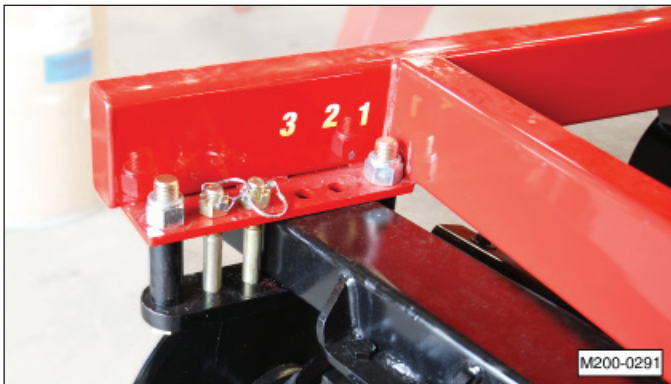
Adjustments for front disk gang.
